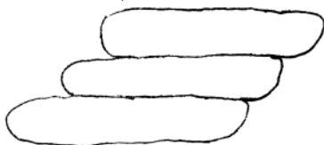
Rounding the underside corners of thinner stone helps to smooth the curve
